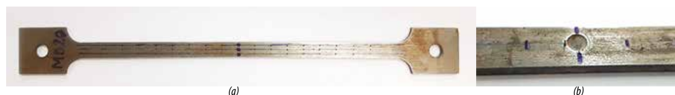
Figure 6. Testing specimens and measuring points (a) and the artificial defect (b).
